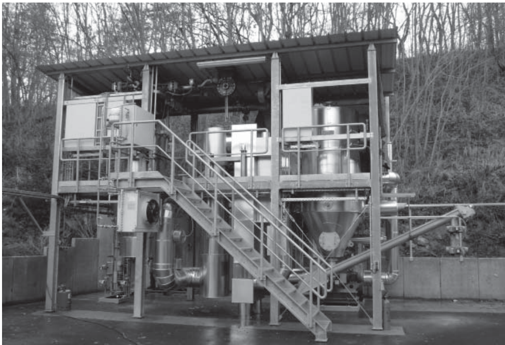
This pilot plant in Gerstungen recovers energy from fine grained production residues. (© Fraunhofer IFF) | Picture in color and printing quality: www.fraunhofer.de/press
