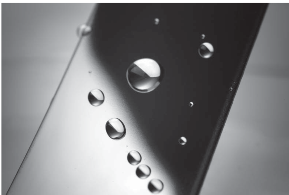
Water droplets on a steel surface with anti-fouling coating. (© Fraunhofer IST) | Picture in color and printing quality: www.fraunhofer.de/press
