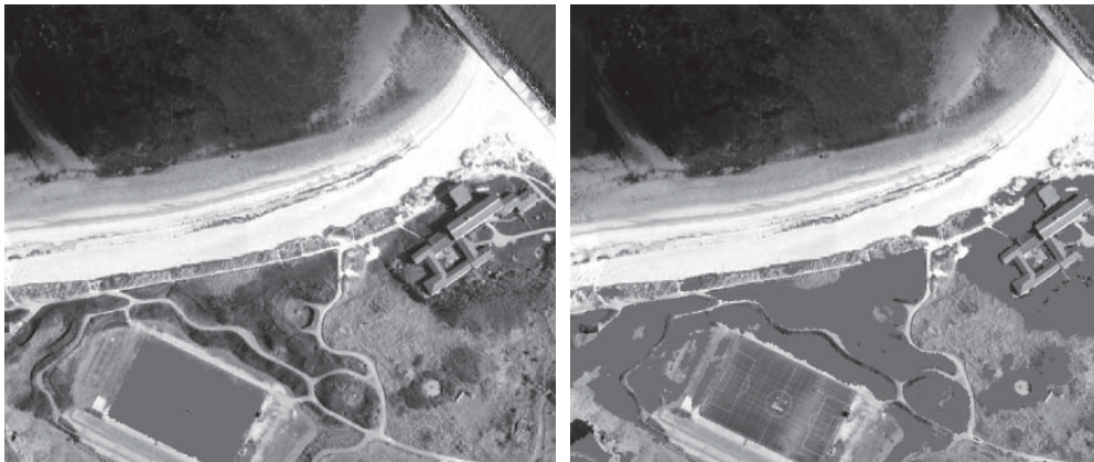
Artificial turf (left) or real vegetation (right)?: The SpectralFinder recognizes the color spectrum of surfaces in real time. (© Fraunhofer IOSB) | Picture in color and printing quality: www.fraunhofer.de/press
