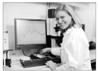
The optical analysis system of IGB: the spectra recorded by the Raman spectroscope (back right) are displayed graphically on a monitor screen. The scientist controls the laser with the small box. (© Fraunhofer IGB) | Picture in color and printing quality: www.fraunhofer.de/ press
