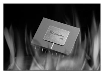
Keeping their cool at 300 °C: the especially compact microchips of Fraunhofer IMS. (© Fraunhofer IMS) | Picture in color and printing quality: www.fraunhofer.de/press
