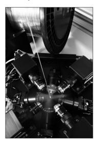
With the WIRE-AOI wire inspection system, four cameras collectively deliver 40,000 analyzed images per second. Thus, a 100% control of the wire surface in real time can also work with very rapid production processes. (© Fraunhofer IPM) | Picture in color and printing quality: www.fraunhofer.de/press
