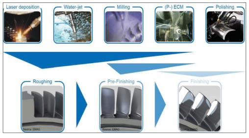
A new study compares different process chains in Blisk manufacturing from an economic and technological point of view. © Fraunhofer IPT | Picture in color and printing quality: www.fraunhofer. de/en/press
