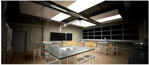
Ceiling-wide activation ensures healthy ambient climate control regardless of the dew point. © Alexander Buff / Fraunhofer IBP | Picture in color and printing quality: www.fraunhofer.de/en/ press
