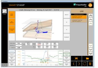
Smart Stamp: a virtual twin of the actual forming press determines the degree of ram tilt. © Fraunhofer IWU | Image in color and print quality: www.fraunhofer.de/en/press.
