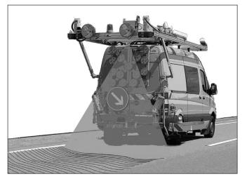
A single laser scanner is all it takes to measure the evenness of a road four meters in breadth with a laser beam. (© LEHMANN + PARTNER GmbH) | Picture in color and printing quality: www. fraunhofer.de/press
