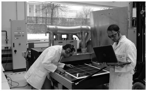
Scientists are laminating a solar cell at CSP in Halle. The process is twice as fast as it used to be. (© Fraunhofer CSP) | Picture in color and printing quality: www.fraunhofer.de/press
