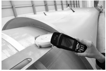
RFID chips in the module and in the locator make automatic continuous tracking possible. (© Dirk Mahler) | Picture in color and printing quality: www.fraunhofer.de/press
