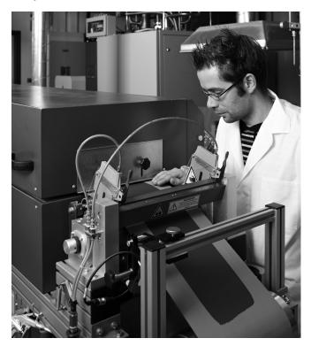
Roll-to-roll coating of electrodes at IWS: The scientists now have optimized the design of anode and cathode for lithium-sulfur batteries. (© Jürgen Leibmann) | Picture in color and printing quality: www.fraunhofer.de/press
