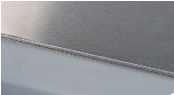
... that allows strong, high-quality joints to be created between steel and aluminum parts. © Fraunhofer IPT
