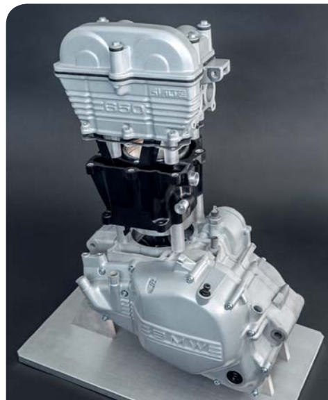
Experimental engine built using the new, lightweight cylinder housing. © Fraunhofer ICT
