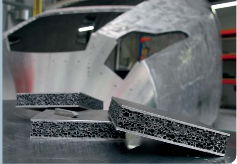
Blue Train: The innovative aluminum foam made it possible to reduce the weight by 20 percent compared to conventionally manufactured locomotives. Tooling costs are cut by 60 percent as well. © Fraunhofer IWU
