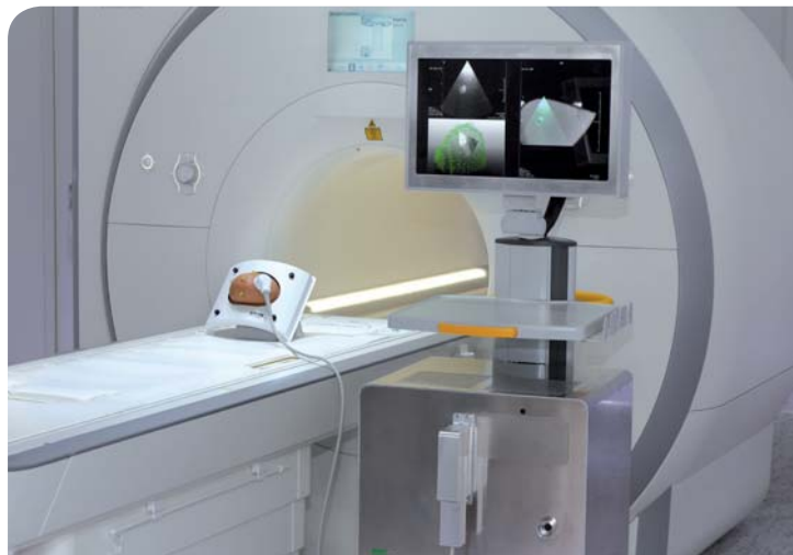
Ultrasound images are recorded during the MRI scan. © Fraunhofer IBMT
