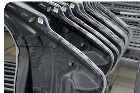
At BMW: the first car with a passenger cell of carbon fiber to be mass-produced. © bimmertoday.de
