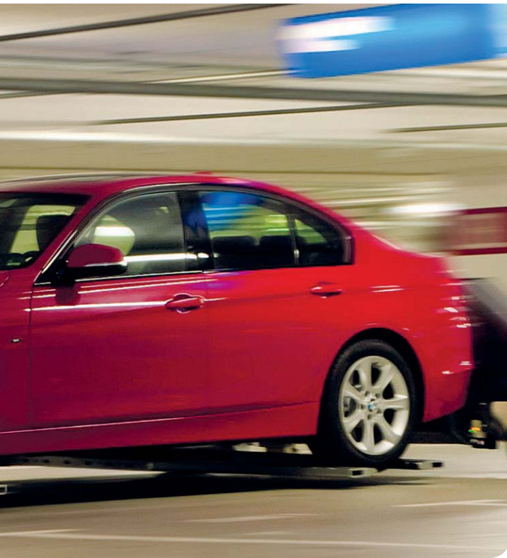
Automated parking using a parking robot. © serva transport systems GmbH
