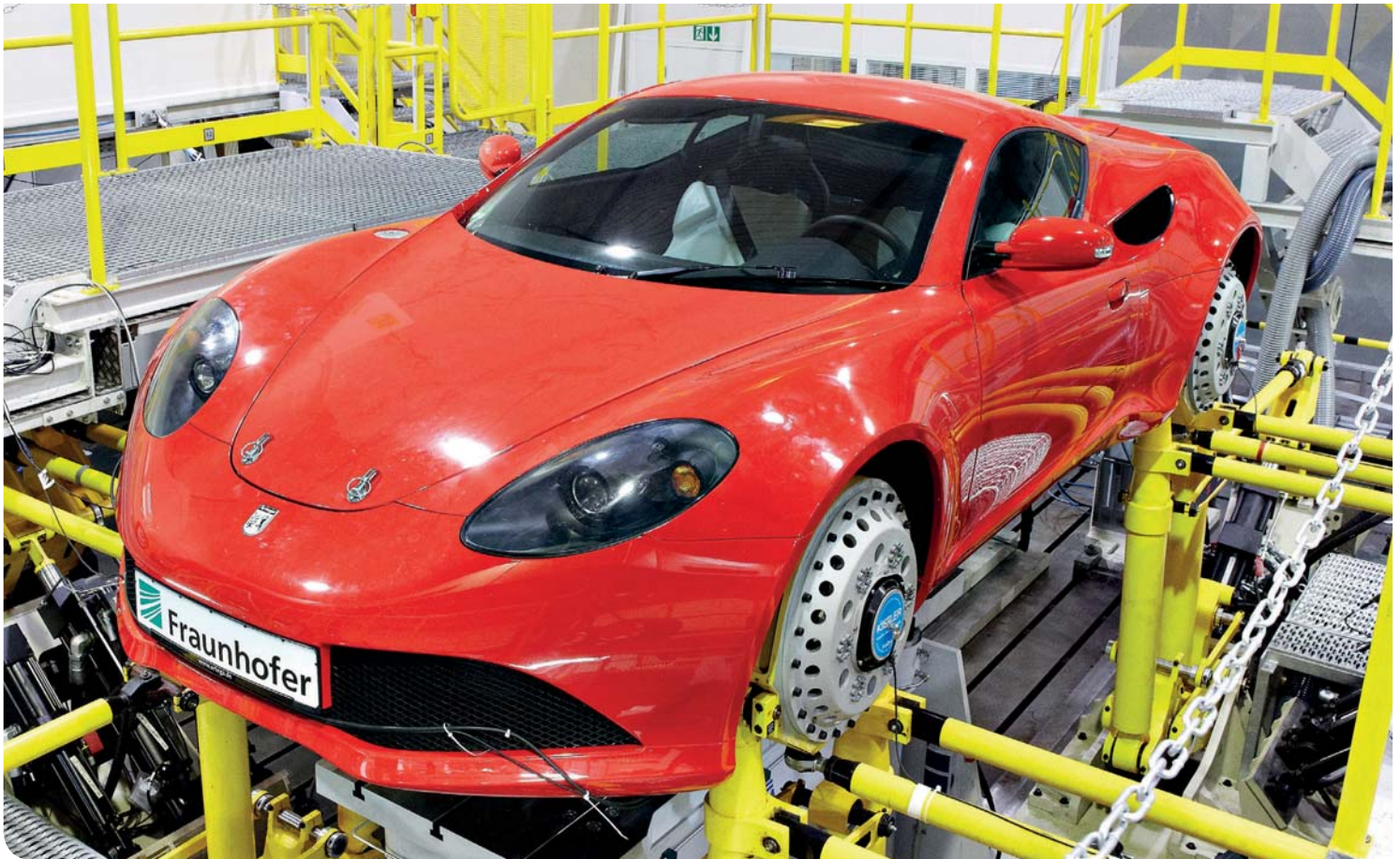
Fraunhofer's Frecco 2.0 e-concept car on the whole-vehicle test rig. © Fraunhofer LBF
