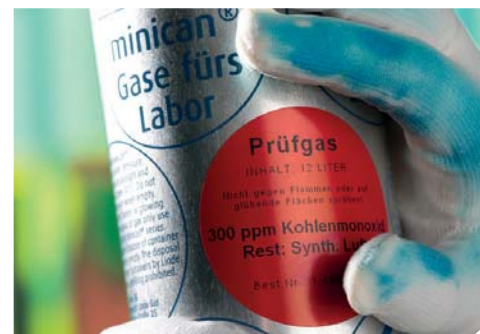
The sensor-fitted glove turns blue when there is a hazardous substance on the container. © Fraunhofer EMFT
