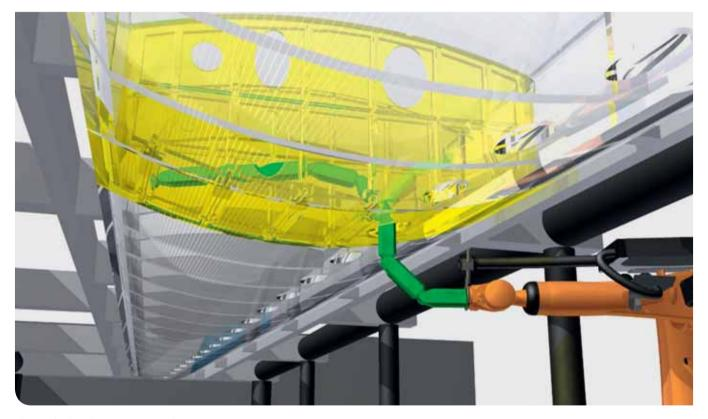
Like a snake the robot can rotate in order to reach the furthest extremities of the wingbox cavities. © *Fraunhofer IWU*
