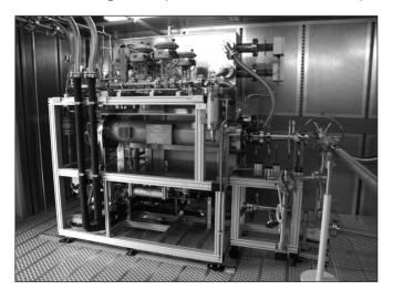
Researchers at a new hot gas test facility are testing the waste heat use systems and turbo-chargers. Their goal is to develop more efficient powertrain concepts for passenger vehicles and trucks. (© Fraunhofer ICT) | Picture in color and printing quality: www.fraunhofer.de/press
