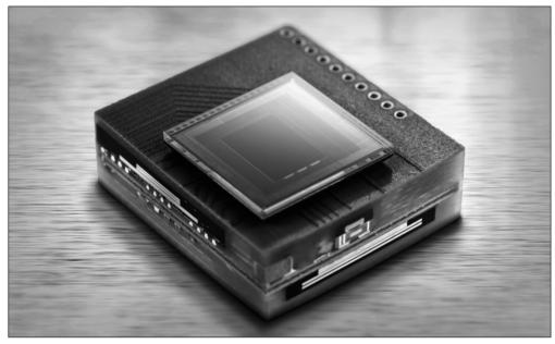
Cross-section of the microcamera module, with the image sensor mounted on the Printed Circuit board. (© Fraunhofer IZM) | Picture in color and printing quality: www.fraunhofer.de/press
