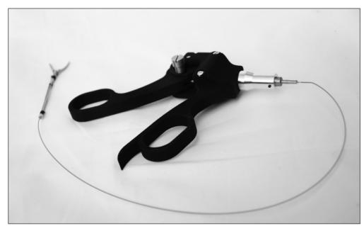
Hydraulic instruments support surgeons when working with endoscopes. The gripping force at their tip is greater. Medicines are able to operate more precisely. (© Fraunhofer IPA) | Picture in color and printing quality: www.fraunhofer.de/press
