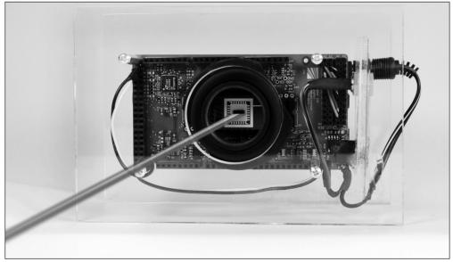
Emission spectrometers analyze materials on the basis of their emitted light spectrum. Novel sensors permit the development of even smaller, faster and more precise test instruments. (© Fraunhofer IMS) | Picture in color and printing quality: www.fraunhofer.de/press
