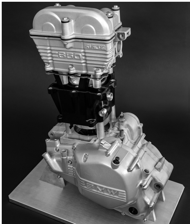
Demonstration model of the experimental engine with lightweight cylinder casing to be presented at the Hannover Messe. (© Fraunhofer ICT) | Picture in color and printing quality: www.fraunhofer.de/press
