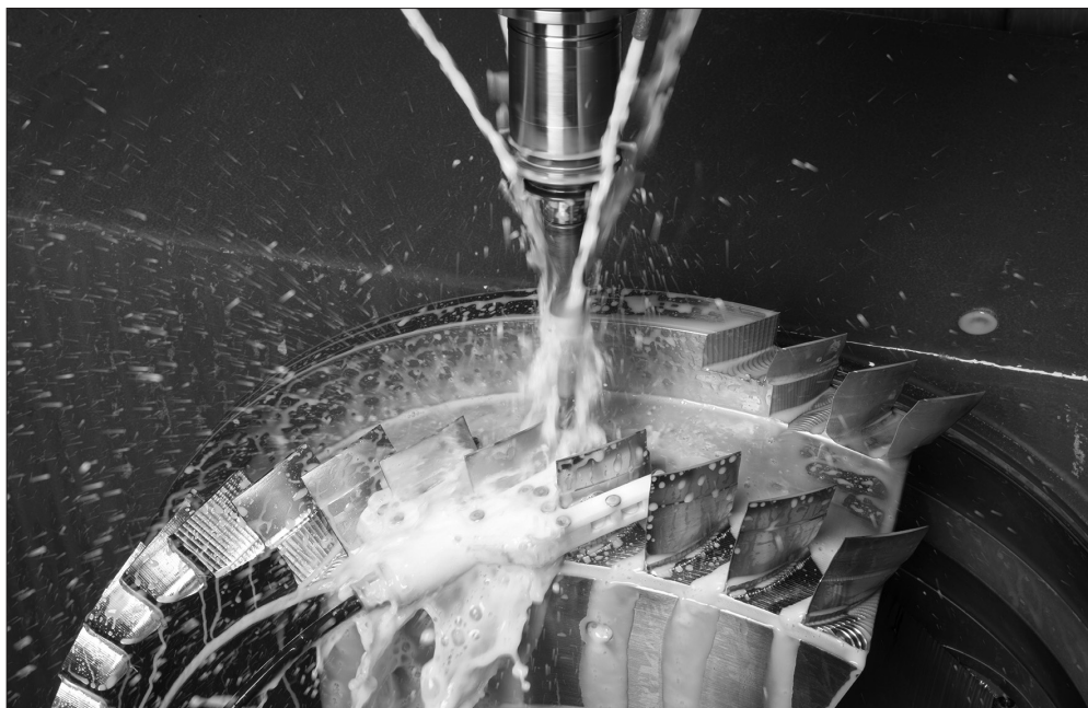
The three-part clamping system holds the blisk blades (just below the middle of the picture in white). Cooling lubricant is being injected from above. (© Fraunhofer IPT) | Picture in color and printing quality: www.fraunhofer.de/press
