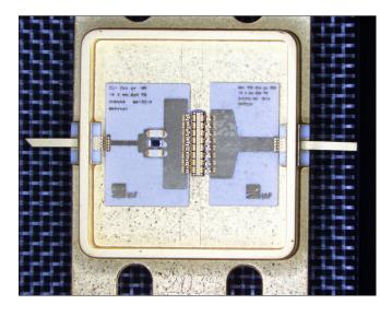
The power amplifier of the Fraunhofer IAF transmits at a frequency of 5.8 gigahertz. These frequency is needed for the new 5G mobile radio standard. The centrally placed gallium nitride (GaN) semi-conductor circuits are the central part of the packaged power amplifier. © Fraunhofer IAF | Picture in color and printing quality: www.fraunhofer. de/en/press
