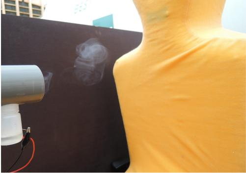
Vortex ring generator prototype. The plan is to integrate the system into the back of passengers' seats. © Fraunhofer IBP | Picture in color and printing quality: www.fraunhofer.de/en/press
