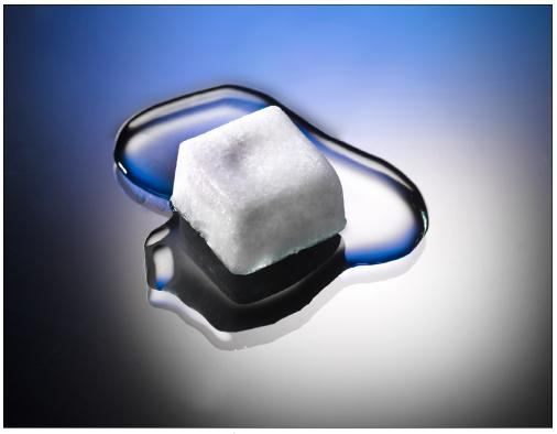
The PCM cube maintains a temperature of 21 degrees Celsius until it is completley melted.
