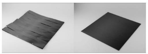
Carbon fibers and heated plastic combine under pressure to form a homogeneous CFRP plate. With infrared radiation in a vacuum, this occurs quickly and with a high degree of energy efficiency.
