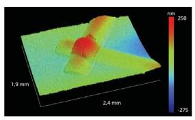
Sealing bars fitted with thin-film sensors (left). White light interferometer image of a measuring point with conducting tracks approx. 250 nm thick and 600 µm wide (right). © Fraunhofer IWM | Picture in color and printing quality: www.fraunhofer.de/en/press.
