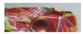
Examples of leaking or visually deficient film packaging: contamination via packaged goods in the sealed seam (above) and folds in the weld seam (below).
