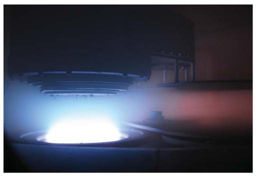
View inside vacuum chamber during the coating process. © Fraunhofer IWM | Picture in color and printing quality: www.fraunhofer.de/en/press
