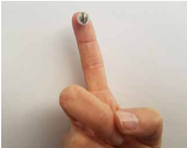
With the miniaturized radio transmission inside the sphere, the measured data is transmitted live to a base station. © Fraunhofer ENAS | Picture in color and printing quality: www.fraunhofer.de/en/press
