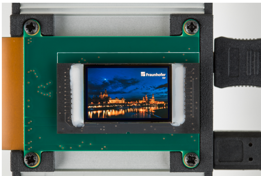
Thanks to a cleverly designed system concept and modern design methodology, the new OLED microdisplay achieves a resolution of 1920 x 1200 pixels. © Claudia Jacquemin | Picture in color and printing quality: www.fraunhofer.de/en/press
