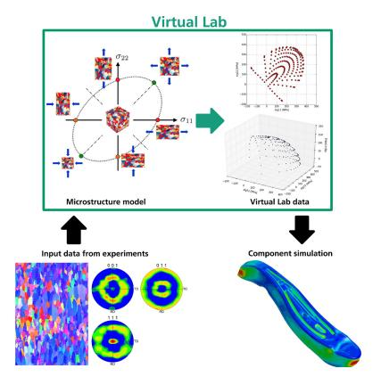
From input data obtained through experiments, via the virtual laboratory, to creation of material cards for component simulation. © Fraunhofer IWM | Picture in color and printing quality: www.fraunhofer.de/en/press
