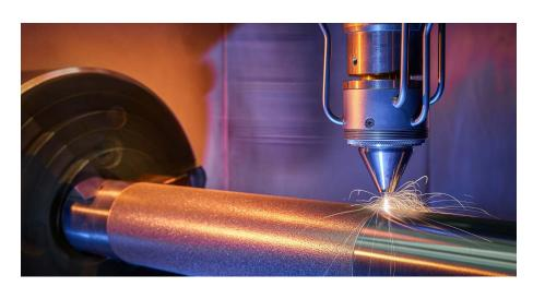
With EHLA, metal protection layers can be applied at an extremely high speed. © Fraunhofer ILT, Aachen/Volker Lannert | mages in color and print quality: www.fraunhofer. de/press/research-news
