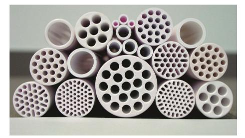
Ceramic membranes by the Fraunhofer Institute for Ceramic Technologies and Systems IKTS. © Fraunhofer IKTS | Images in color and print quality: www.fraunhofer.de/press/ research-news
