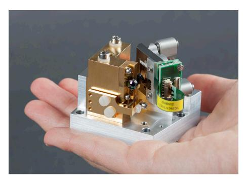
Demonstrator of the miniaturized laser source consisting of a quantum cascade laser chip and a MOEMS grating scanner. © Fraunhofer IAF | Picture in color and printing quality: www.fraunhofer.de/en/press
