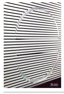
Prototype sheet glass with curvatures on both sides: the flat areas are undistorted and free of pressure marks. © Fraunhofer IWM, Foto: Felizitas Gemetz | Picture in color and printing quality: www.fraunhofer. de/en/press
