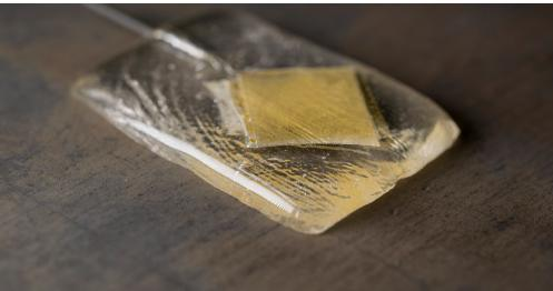
High-temperature ultrasonic transducer. © Katrin Selsam-Geißler / Fraunhofer ISC | Picture in color and printing quality: www.fraunhofer.de/en/press
