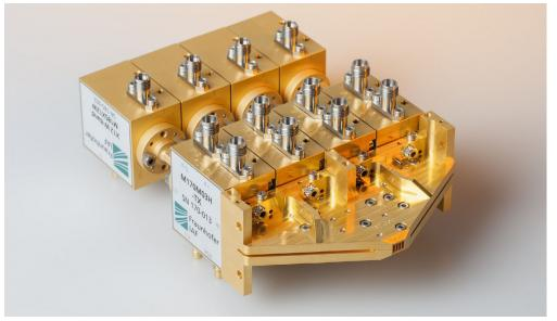
In the TERRANOVA project, Fraunhofer IAF is focusing on the integration of wireless modules at the chip level. The image shows a functional prototype of a 300 GHz multichannel wireless system for further integration as a system-on-chip. © Fraunhofer IAF | Picture in color and printing quality: www.fraunhofer.de/en/press
