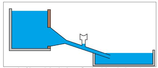
Cross section of the Venturi tube. When the water flows through the uptake tube, negative pressure builds that forces the elastomer film (center of the image) to extend inwards.
