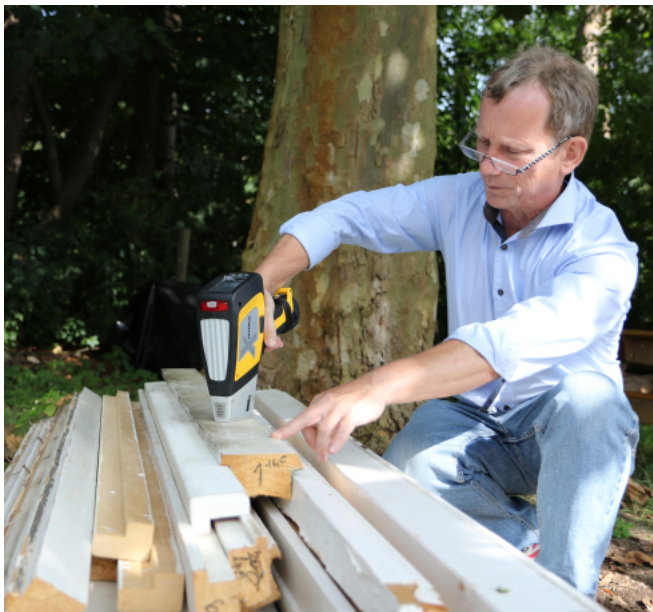
Physicist using a hand-held X-ray fluorescence to test sections of salvaged window scantlings for the presence of inorganic wood preservatives. © Fraunhofer WKI/Simone Peist | Picture in color and printing quality: www.fraunhofer.de/en/press
