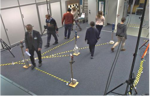
Lab testing at Fraunhofer FKIE to see how robust the security assistance system is: it must be able to clearly identify the carrier of a dirty bomb without sounding a false alarm. © Fraunhofer FKIE | Picture in color and printing quality: www.fraunhofer.de/en/press
