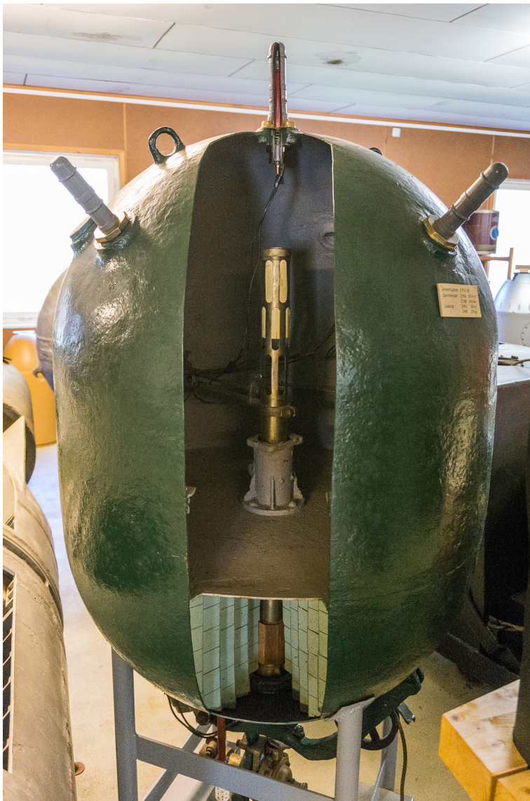
Disassembled moored mine. © Schleswig-Holstein ordnance disposal team teaching materials
