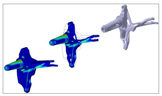
Finite element analysis of the start design of a wheel bearing technology demonstrator (left); numerical design optimization of the technology demonstrator to reduce the component's mass without impairing functionality (center); and CAD template for manufacturing the 3D metal component (right).© Fraunhofer EMI | Picture in color and printing quality: www.fraunhofer.de/en/press
