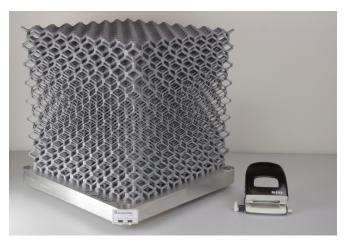
Lattice cube with edge length of 40 centimeters, one of the largest metal structures manufactured using selective laser melting (SLM). © Fraunhofer EMI | Picture in color and printing quality: www.fraunhofer. de/en/press
