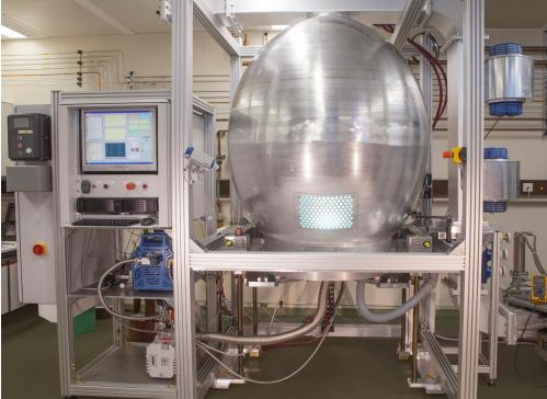
The special ellipsoid form of the plasma reactor developed at Fraunhofer IAF allows for large-scale diamond separation. © Fraunhofer IAF / Iselin | Picture in color and printing quality: www.fraunhofer.de/en/press
