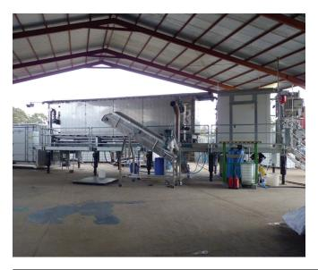
The pilot facility consists of a container with a storage bin and energy center, as well as of a frame that houses the drying and torrefaction reactors, the attachment for extracting solids and the condensers. © Fraunhofer IGB | Picture in color and printing quality: www.fraunhofer.de/en/press
