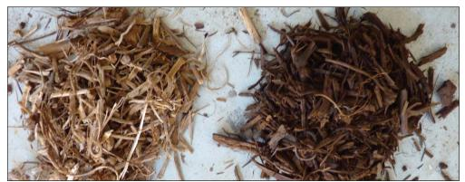
The project partner in Spain is investigating the torrefaction of various lignocellulosic substrates, including pruning (left untreated, right torrefied). © Fraunhofer IGB | Picture in color and printing quality: www.fraunhofer.de/en/press
