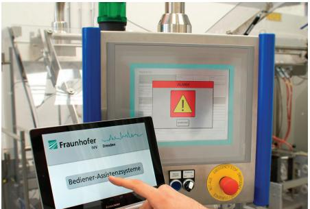
SAM, a self-learning assistance system, helps machine operators resolve errors in production machines. © Fraunhofer IVV | Picture in color and printing quality: www.fraunhofer.de/en/press
