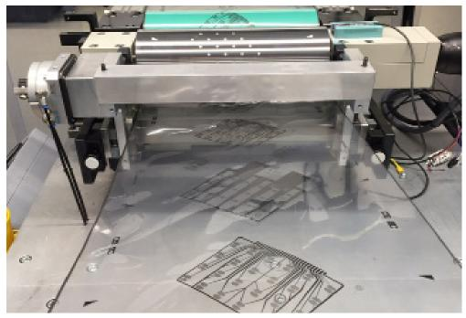
Endless film with printed biosensors: Fraunhofer has developed a convenient roll-to-roll process. © Fraunhofer IBMT | Picture in color and printing quality: www.fraunhofer.de/en/press
