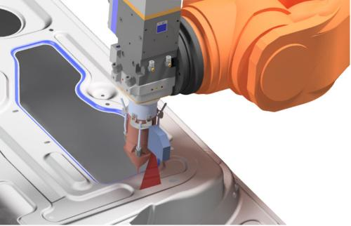
Conventional sensors limit the directional flexibility of robots © Fraunhofer IAPT | Picture in color
