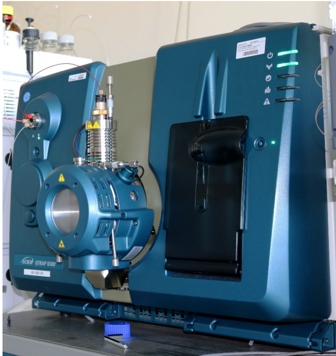
Picture 1: The tandem mass spectrometer is used to separate various substances in tear fluid and determine their concentration.
