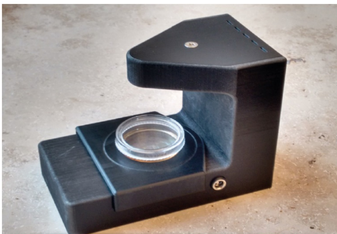
Picture 1: The holographic microscope enables automatic, three-dimensional tracking of immune cells in real time.
