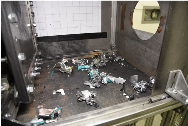
Picture 3: Fragments of a drone battery following impact with an aluminum plate on the test bench.
