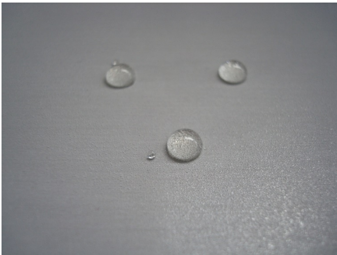
Picture 2: Drops of oil on a super hydrophobic and oleophobic coating on stainless steel.
