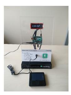
Picture 1: AIfES demonstrator for handwriting recognition. Numbers written by hand on the PS/2 touchpad are identified and output by the microcontroller.
