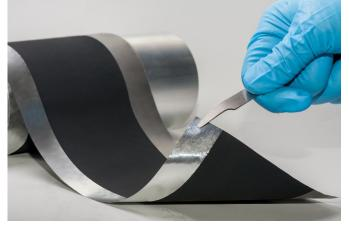
This is what the electrodes coated with the new dry transfer coating technology look like. Fraunhofer IWS process enables battery electrodes to be produced on a pilot scale without using toxic solvents.
