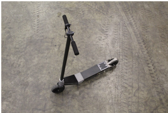
Fig.1 Hybrid metal and carbon fiber reinforced plastic e-scooter
