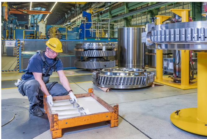
Fig. 1: ErgoJack with a locking hip joint and leg brace supports the worker when lifting heavy loads.
