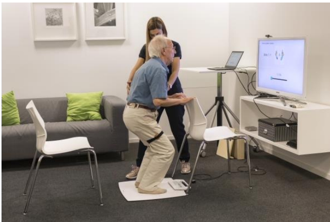
Fig. 1 Training with instructions: after analyzing movements, AICOS software creates an individual movement profile and assesses the risk of falling.
