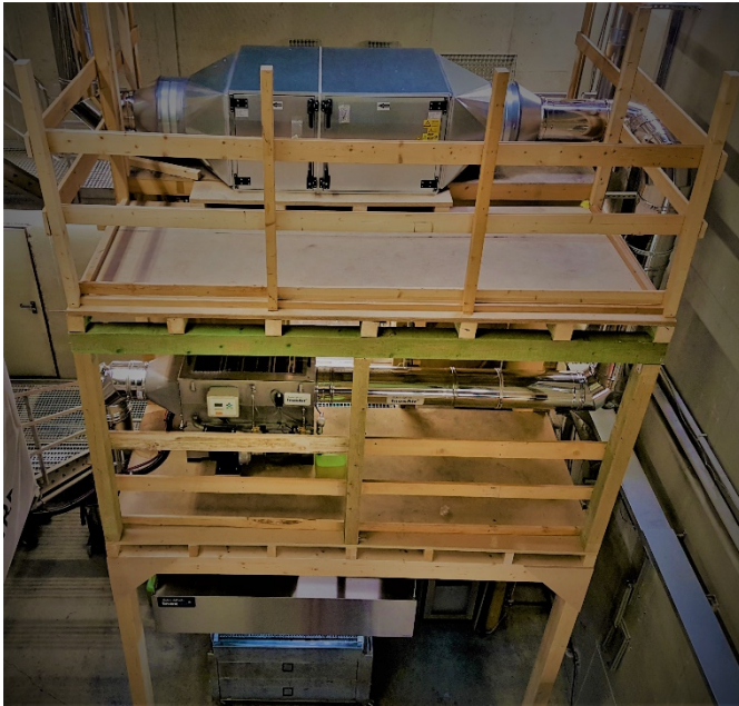
Picture 1: To carry out their experiments, the researchers set up a commercial grill in the institute's laboratory – including a meter-high exhaust air treatment system.
