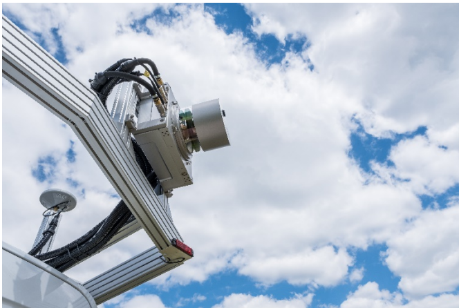
Picture 1: 3D laser scanner contained in a housing and mounted on the roof of a vehicle.
