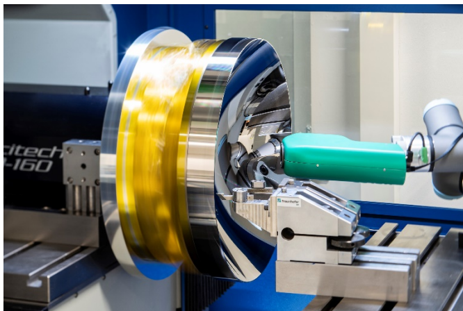
Picture 2: Roughness inspection during diamond turning with a light scattering sensor
