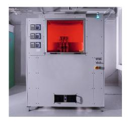
Fig. 1 System for Multi Material Jetting of highperformance components with combined properties or functions.
